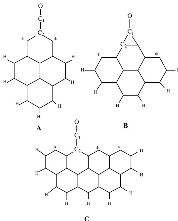
**Figure 1.** Geometry of the carbonyl models selected. (\*) Active sites.
